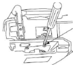
Chain oil flow adjusting
